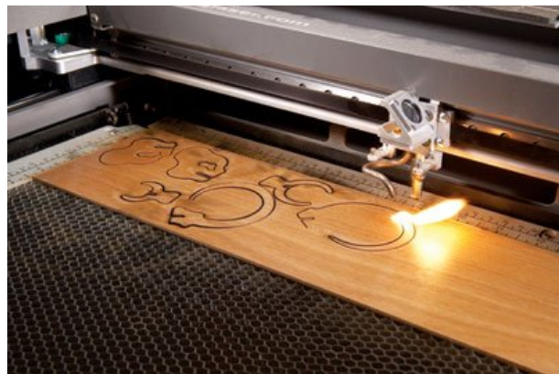
Figure 1: Wood cutting by laser [1].
